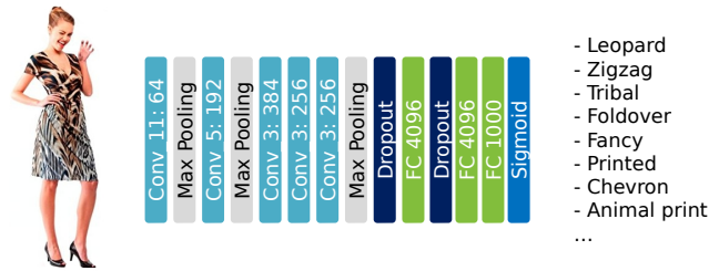
Figure 2: The architecture of our deep attribute CNN model.
