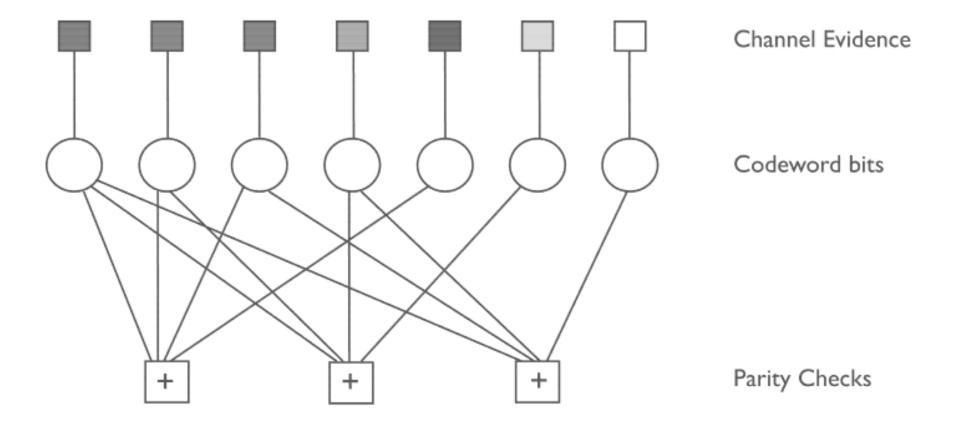
A factor graph for (N=7,k=3) Hamming code, which has 7 codeword bits, of the left-most four are information bits and the last 3 are parity bits.
