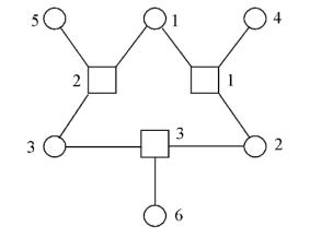
We have transmitted N = 6 bits with k = 3 parity check constraints.
