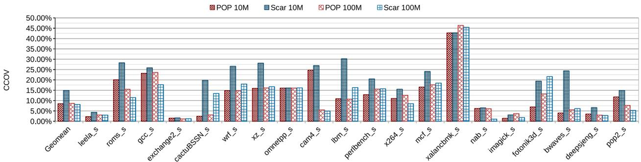
Fig. 9. Corrected Coefficient of Variation (CCoV) metric for Spec2017 Speed benchmarks, Reference Dataset.
