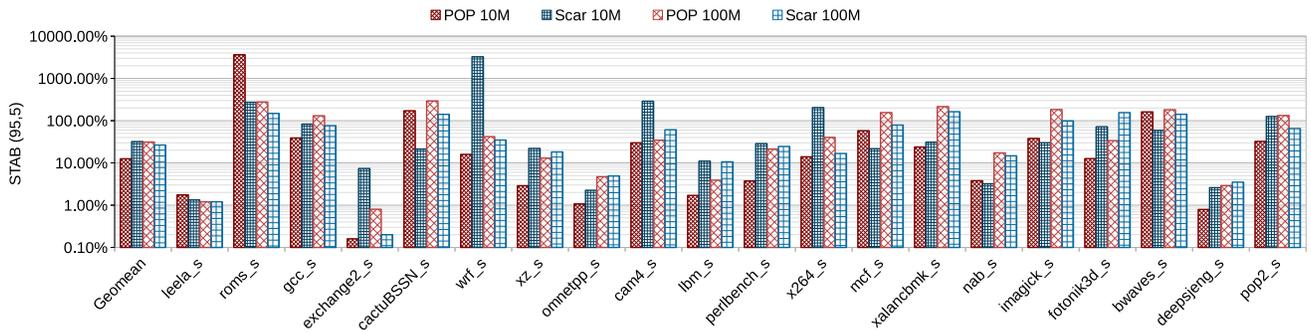
Fig. 10. Normalized STAB<sub>95,5</sub> metric for Spec2017 Speed benchmarks, Reference Dataset.
