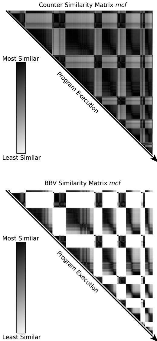
Fig. 4. Similarity matrices show the similarity between interval signatures, where the diagonal of the matrix represents the program’s execution. A darker color indicates greater similarity, as measured by percentage distance. We show the similarity matrix for counters (top) and BBVs (bottom) for the Spec2006 *mcf* benchmark.
