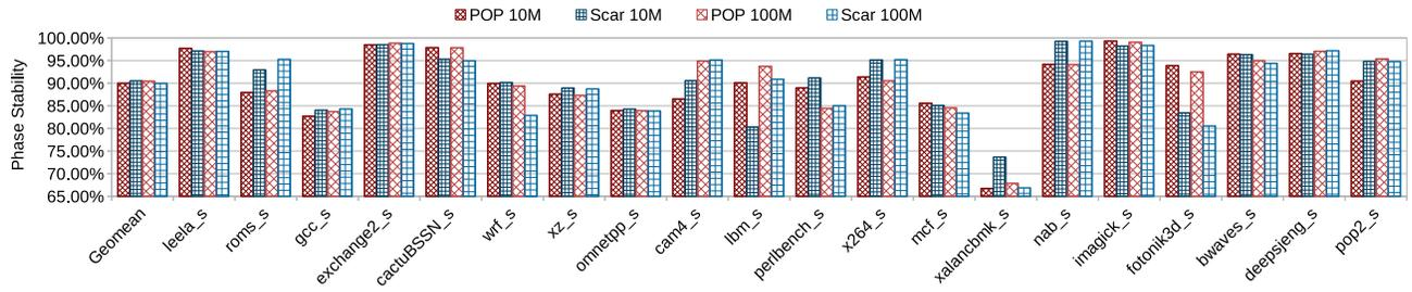
Fig. 7. Phase Stability metric for Spec2017 Speed benchmarks, Reference Dataset.
