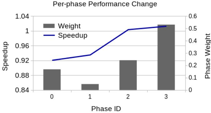
Fig. 2. The `lbm_s` performance change (denoted by the S-Curve) per phase via disabling spatial L2 prefetcher, with respective phase weights denoted by bars. The phase weight refers to the amount of time the program spends in a particular phase, relative to the program as whole. As a result, the sum of phase weights is always 1.
