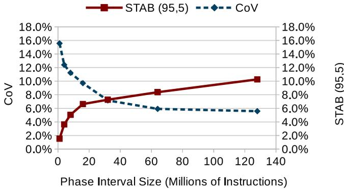
Fig. 5. Trade off between CoV and STAB using various interval sizes. While CoV suffers at smaller intervals, many more intervals are available for analysis. As a result, the STAB overhead reduces at smaller intervals.
