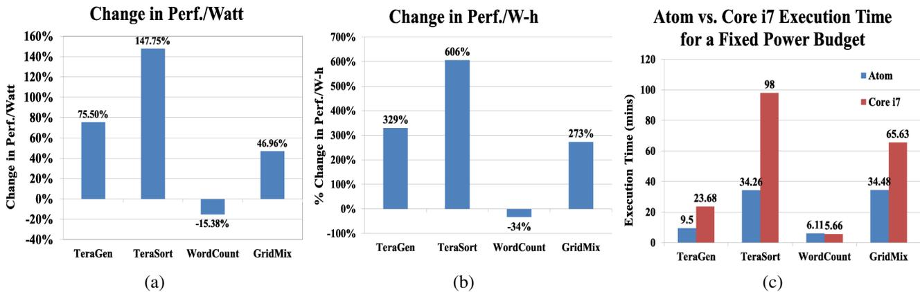
Figure 8. Change in Perf./Watt, Perf./W-h, and Execution Time on the System Compared to Core i7 Cluster in a Fixed Power Budget
