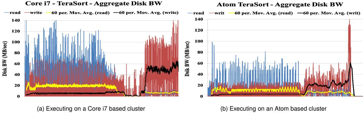
**Figure 2.** Disk bandwidth utilization by Core i7 and Atom based clusters while executing TeraSort benchmark. The overlaid lines are 1 minute averages of individual data points.
