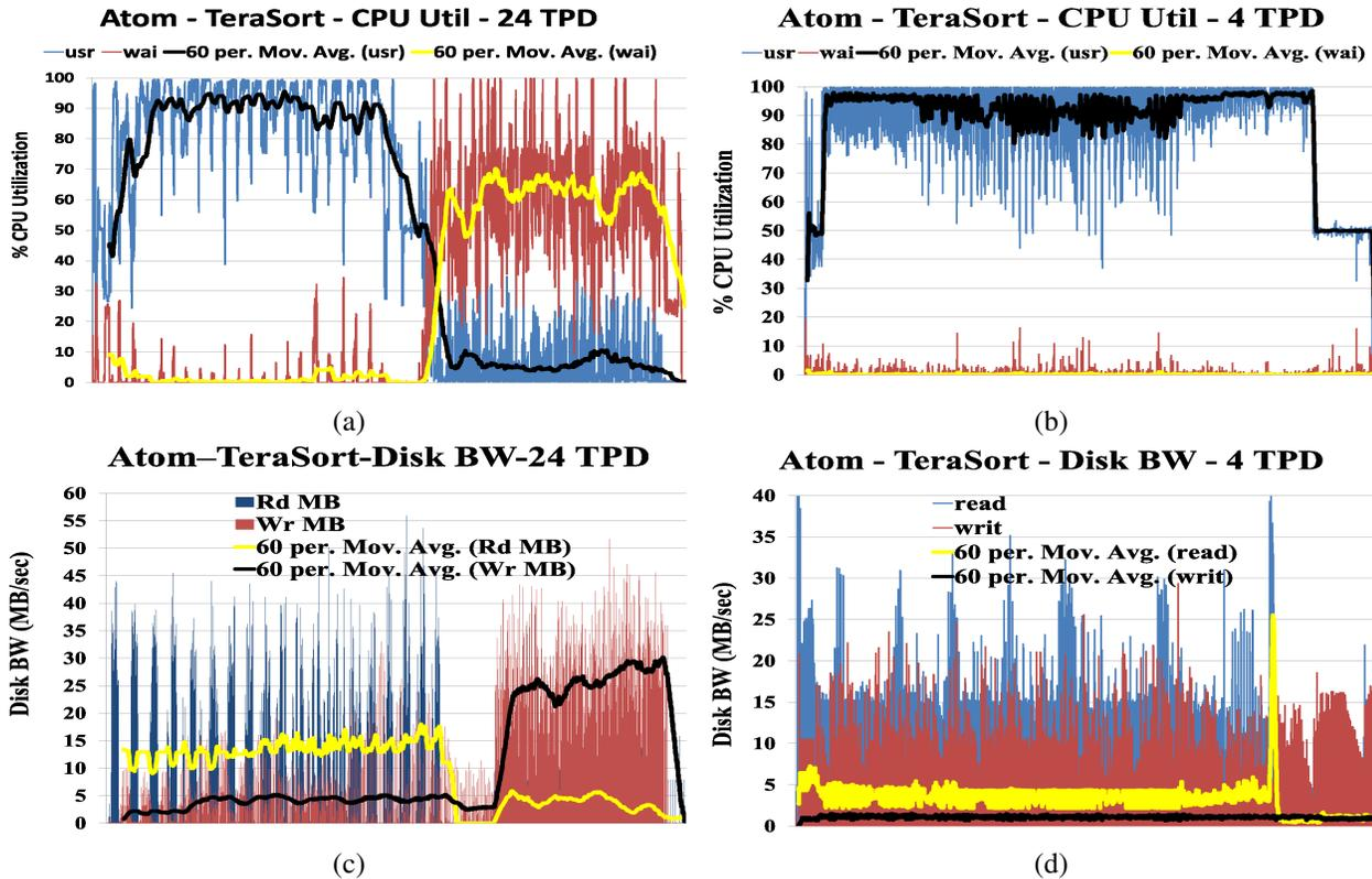
Figure 10. CPU and Disk Utilization for the Best and Worst Execution Time on the System.
