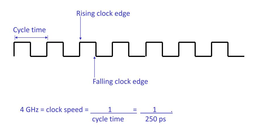
Until now, circuits were combinational – when inputs change, the outputs change after a while (time = logic delay thru circuit)
