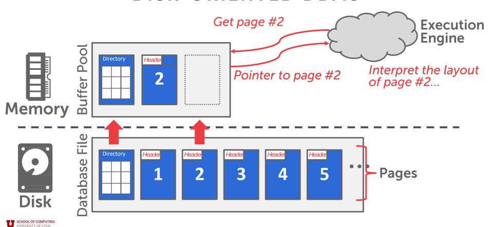
The DBMS can use memory mapping (mmap) to store the contents of a file into the address space of a program.
