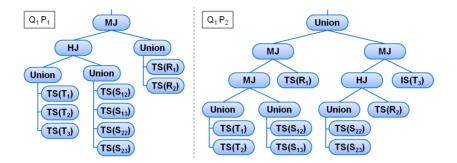
**Figure 2.4:**  $Q_1P_1$  and  $Q_1P_2$  are plans that can be generated by optimizers in parallel database systems for our example query  $Q_1$ . IS and TS are respectively index and table scan operators. HJ and MJ are respectively parallel join operators based on hash and merge. Union is a bag union operator.
