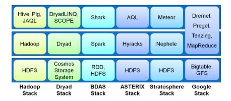
Figure 5.1: Typical dataflow software stacks along with the Hadoop stack.
