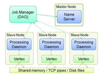
Figure 5.2: Dryad system architecture.
