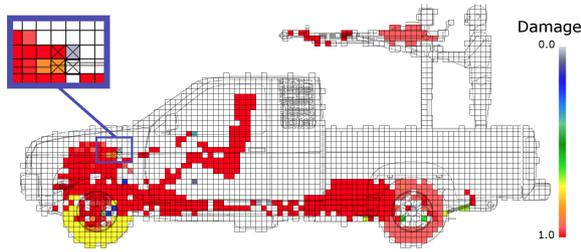
**Figure 3:** A cell plot output from ballistic simulations. Cell color encodes the quantitative damage that each shot inflicts on this vehicle's mobility or firepower capabilities. Analysts understand cell plots by comparing cells to their neighbors of different colors, such as the highlighted cells marked here.
