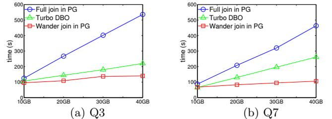
**Figure 5: Experimental results with limited memory, 4GB memory (Wander join in PG and Turbo DBO run to 1% confidence interval).**
