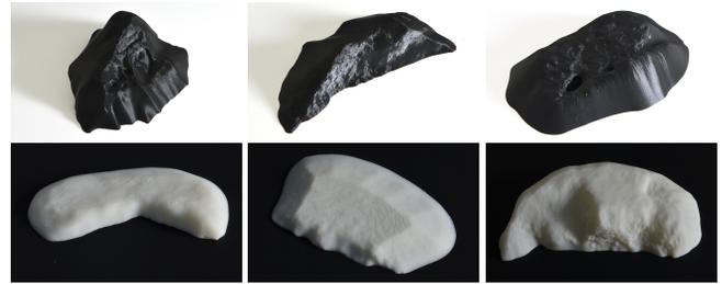
Figure 7. 3D printed holds. Geometry generated by reconstructions from natural rock formations. (Top) “Pilgrimage” route. (Bottom) “TATAN” route.
