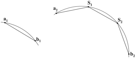
Figure 2: Spherical arc  $\mathbf{a}_1, \mathbf{b}_1$  can be approximated linearly with sufficient accuracy. The same level of accuracy can be obtained even for arc  $\mathbf{a}_2, \mathbf{b}_2$  by using piecewise linear approximation with two samples ( $S_1, S_2$ ) of the original curve.
