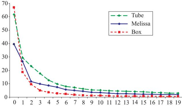
Figure 8: Enveloping error (vertical axis) vs. number of blend bones (horizontal axis).
