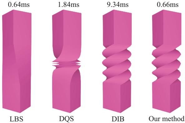
Figure 9: Bending box rotated by nearly 360 degrees. Our method provides an efficient linear approximation of the correct solution (DIB).
