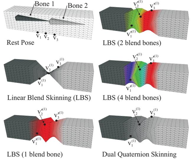
Figure 3: Simple skinned model in the rest pose (top left) and after twisting Bone 2 by 180 degrees (using several different methods).
