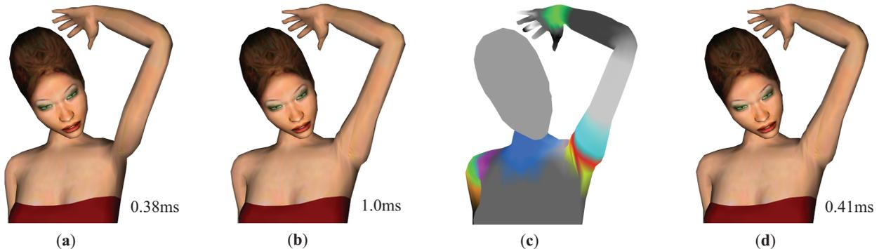
Figure 1: Linear blending is one of the fastest skinning methods, but suffers from volume-collapsing artifacts (a). These artifacts can be removed by a nonlinear blending method (such as dual quaternions), but at the cost of more complex vertex processing (b). Our method automatically places virtual bones in critical parts of the model (c), so that linear blending using these virtual bones efficiently approximates the nonlinear skinning technique (d).
