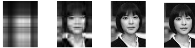
Figure 4: From left to right: only keep the first term; keep the first five terms; keep the first twenty terms; keep the first fifty terms
