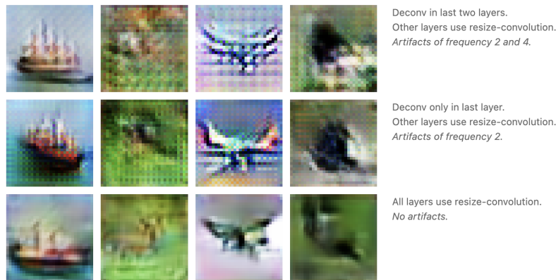
Figure 21: Simply switching out the standard deconvolutional layers for nearest-neighbor resize-convolution causes artifacts of different frequencies to disappear. [Odena et al., 2016]
