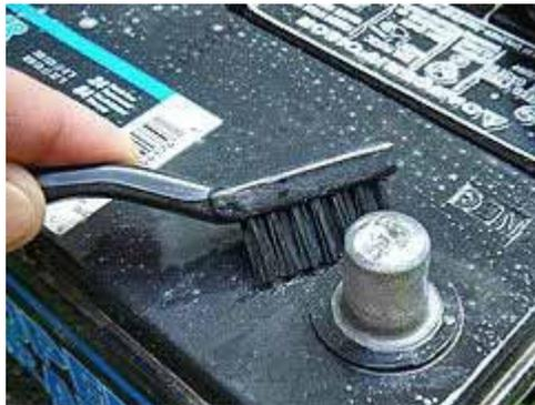
nals is dangerous stuff. It can burn skin and eyes. It's recommended that rubber gloves, long sleeved shirt and eye covering be worn when removing corrosion build up from batteries.
