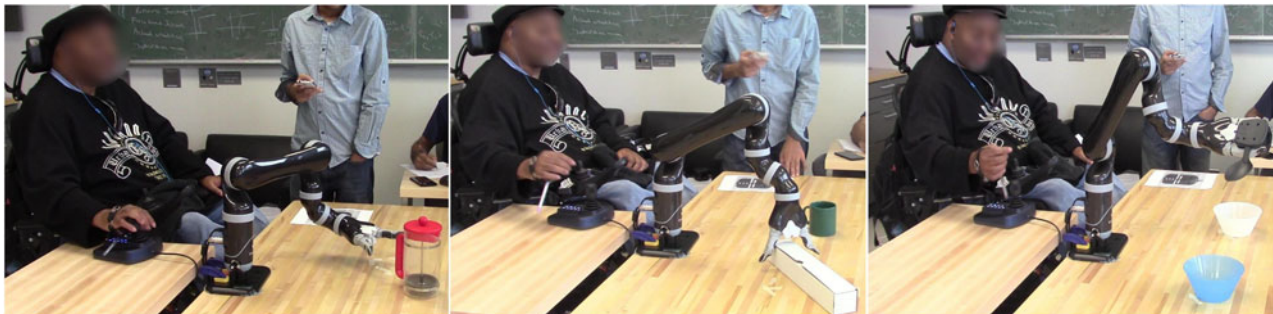
Fig. 3. Study tasks performed by SCI participant. Left to right : Simple Reaching (R), Reaching for Grasping (RfG), Reaching for Scooping (RfS).
