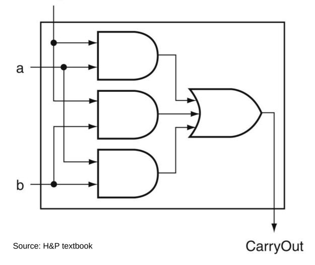
Equations: Sum = Cin  $\overline{A}$   $\overline{B}$  + B.  $\overline{Cin}$  + A.  $\overline{Cin}$ .  $\overline{B}$  + A.B.Cin  $Cout = A \cdot B \cdot Cin +$ A . B . Cin + A. Cin.  $\overline{B}$  + B. Cin. A = A . B +A. Cin +B.Cin
