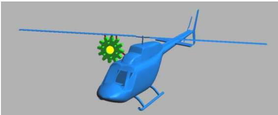
Figure 1: Our system can haptically render models like a 6,000 triangle gear model and a 113,000 triangle helicopter model.
