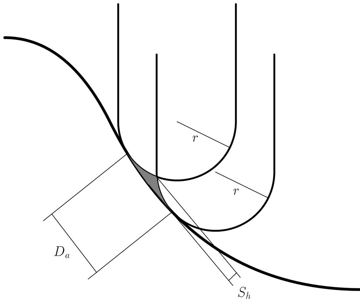
Figure 1: Given the tool radius,  $S_h$  can easily be derived from  $D_a$ .
