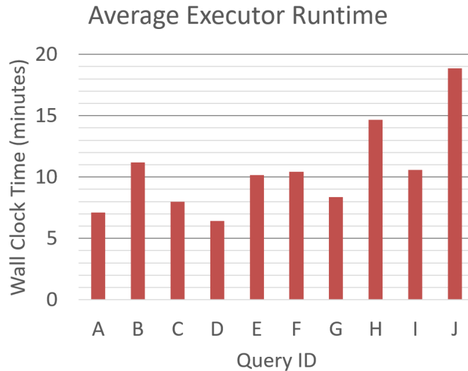
Figure 7: The average wall clock execution time of executor processes. While we capture an initial notion of system state, it is unlikely that the state remains consistent for the entirety of the executor, leading to poor predictions.
