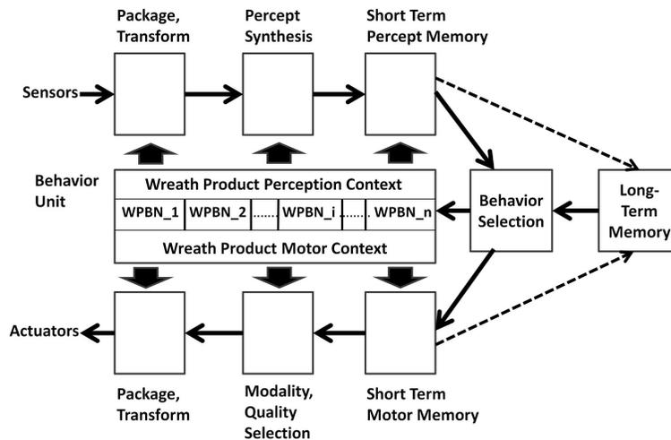
Figure 5: Lower Level Layout of Cognitive Process.
