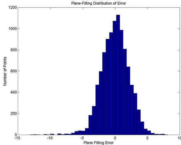
Figure 13: Error Distribution in Plane-Fitting for Kinect Data.
