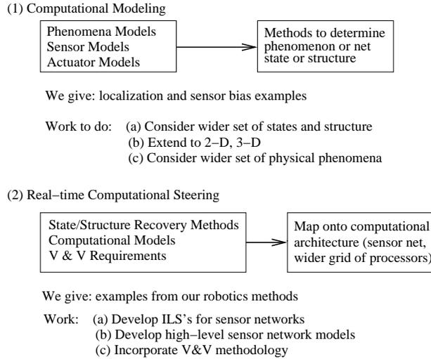
Figure 2: *Computational Sensor Network System Development Framework.*
