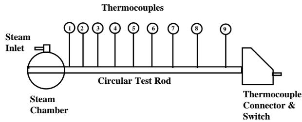
Figure 8: Layout of the Heated Rod Experiment.
