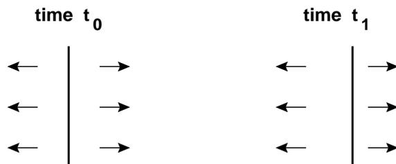
Figure 3: The surface to the left has an optical flow different from that of the boundary and hence is an *occluded* surface. Since it is moving away from the boundary, it is in fact being *disoccluded*.
