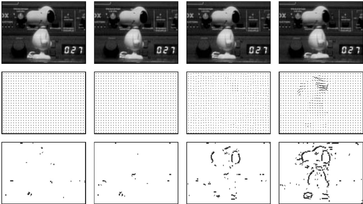
Figure 15: Image sequence, estimated flow, boundary classifications: moving object with near-homogeneous surface.
