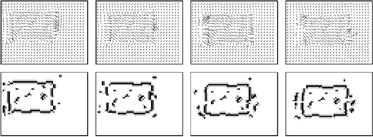
Figure 8: Flow estimation using Horn and Schunck with explicit boundary detection (first four frame pairs).
