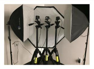
Fig. 3 Our recording setup, featuring three tripod-mounted GoPro cameras and diffuse light sources
