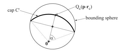
Figure 6.3: If the cap C' centered in the origin has apex  $Q_c(\mathbf{p} - \mathbf{r}_c)$  and angle  $\alpha$ , then its minimal enclosing sphere has center  $\cos(\alpha)Q_c(\mathbf{p} - \mathbf{r}_c)$  and radius  $\sin(\alpha)\|\mathbf{p} - \mathbf{r}_c\|$ .
