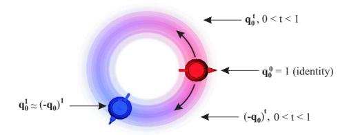
Figure 2.2: Quaternion antipodality. In this example, transformation of the teapot by  $\mathbf{q}_0^t$  for  $t \in [0, 1]$  produces a counterclockwise rotation (longer trajectory), while transformation by  $(-\mathbf{q}_0)^t$  leads to a clockwise one (shorter trajectory).
