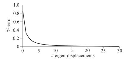
Figure 7.6: The cloth hippopotamus animation (with 100 proxy-joints and rigid transformations) is improved by adding eigen-displacements (Section 7.3). Even one eigendisplacement adds most fine details.
