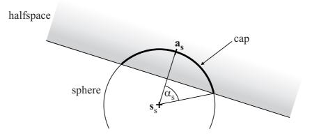
Figure 6.1: Example of a cap in  $R^2$  with center  $\mathbf{s}_s$ , apex  $\mathbf{a}_s$  and angle  $\alpha_s$ . In this case the cap is just a spherical arc.
