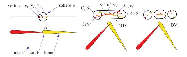
Figure 5.1: Left: the reference posture; middle and right: the animated posture.  $C_{j_1}$   $(C_{j_2})$  is the transformation matrix of joint  $j_1$   $(j_2)$ . Bounding volume  $BV_1$  is bigger than necessary, because it encloses all possible deformations of vertices  $\mathbf{v}_1, \mathbf{v}_2, \mathbf{v}_3$ . Our algorithm uses an optimized bounding volume  $BV_2$ , which considers actual vertex weights.
