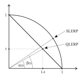
Figure 3.4: Difference between the QLB angle  $\alpha(t)$  and the SLERP one,  $\beta(t)$
