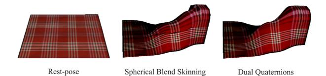
Figure 4.1: Piece of cloth deformed by spherical blend skinning reveals artifacts caused by discontinuous change of rotation centers. Dual quaternion skinning (Section 4.5) does not have such problems and produces a smooth deformation.
