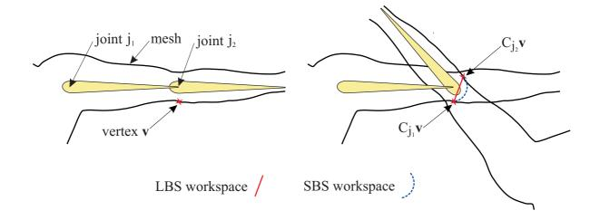
Figure 3.2: The set of possible results of LBS is a line segment, while SBS gives a circular arc.
