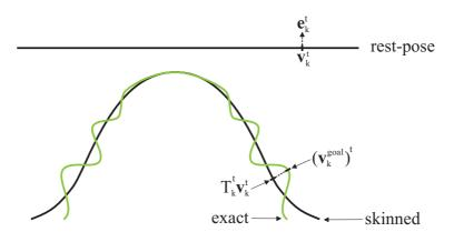
Figure 7.3: Differences between the exact mesh position,  $(\mathbf{v}_k^{goal})^t$ , and its skinning approximation,  $T_k^t \mathbf{v}_k^t$ , are mapped to the rest-pose, and denoted as  $\mathbf{e}_k^t$ .
