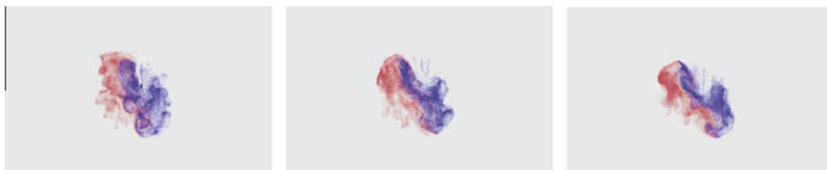
Fig. 5. Smoke ball collision simulations using linear scheme (left), mono Catmull–Rom (middle), and adaptive Catmull–Rom interpolations (right) [21].
