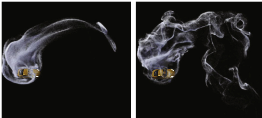
Fig. 7. Smoke simulations with the semi-Lagrangian (left) and the modified MacCormack methods (right) [17].
