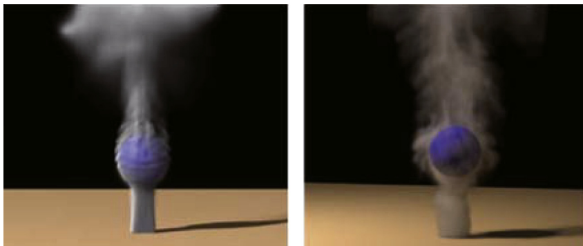
Fig. 1. Visual comparison of smoke simulations using octree grid (left) [3] structure and MAC (right) [7].
