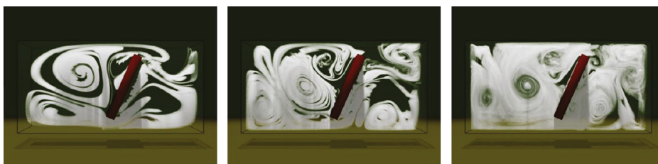
Fig. 8. Simulations using the semi-Lagrangian advection (left) and the QUICK advectations with low- and high-resolution grid configurations [26].
