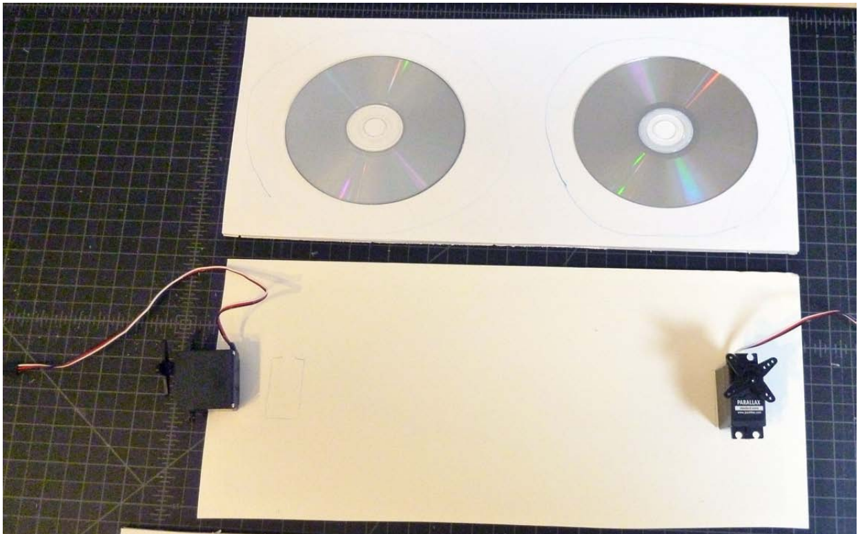
Figure 13: Here I've drawn around the servos with a pencil to mark where I'll cut the holes in which the servos will be placed. I've also used CDs as a rough guide to drawing circles for the drive disks. Note that the drive disks don't have to be perfectly round unless you want them to be. Non-roundness won't impact their function.
