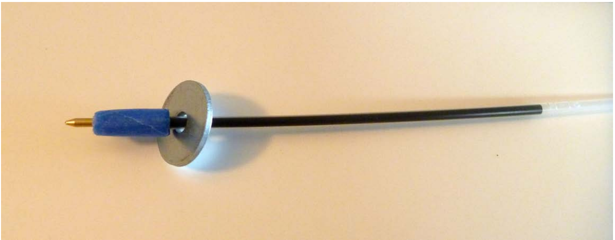
Figure 23: I need a flat surface for the foam core to pivot on. I've made a "shelf" using masking tape, and then put a fender washer (a washer that is a little larger in diameter than a standard washer) on the pen. The foam core will ride on top of this fender washer.
