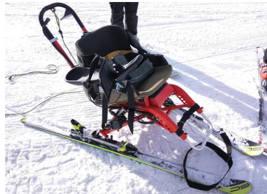
Figure 1. Tetra-Ski. Adaptive skiing equipment.
