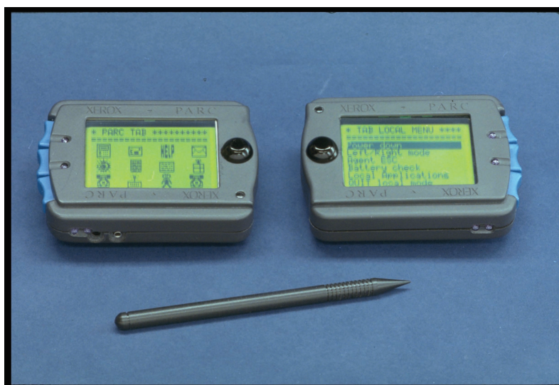
Figure 1. A ParcTab, the inch-scale computer that Weiser foresaw sprinkled in offices by the hundreds. (Photo courtesy of Palo Alto Research Center, PARC; http://www.parc.com .)
