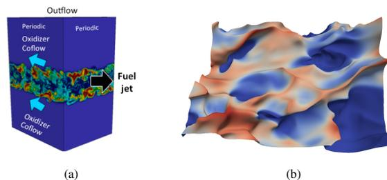
Figure 1: (a) Schematic of the DNS domain for the turbulent jet flame. Image courtesy of [4]. (b) The jet flame isosurface of mixture fraction with interpolated OH concentration. The ‘blue’ regions represent extinction regions and ‘red’ indicates an active chemical process. The isosurface is complex and can fold on itself making feature tracking challenging.
