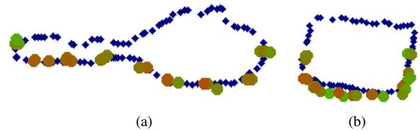
Fig. 6: Visualization of ground truth pushing scores for the large brush and soap box. Green points represent better scores, while redder represent worse.
