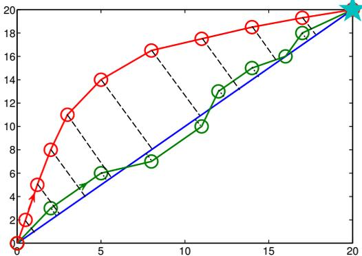
Fig. 3: Two synthetic push trajectories going from initial location in the bottom left to the goal location (star) in the top right. The red trajectory receives a push-stability score of 3.94cm while the straighter green trajectory receives a score 0.62cm.
