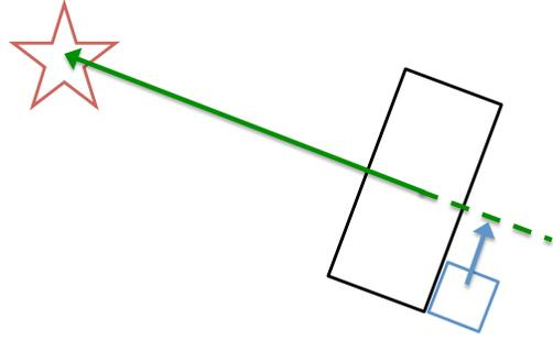
Fig. 4: Visualization of the feedback control policy. The green arrow depicts the goal oriented term of the controller from the object centroid to the goal (red star). The blue arrow show the term used to align the end effector (blue) with the center of the object. These two vectors are scaled and combined to create the commanded velocity of the end effector.
