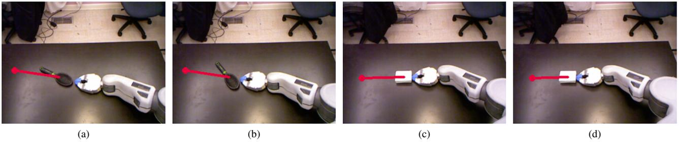
Fig. 1: Example pushing instances. The first two images are two consecutive frames captured while the robot pushes the large hair brush from an unstable pushing location. The second two frames show the robot pushing a soap box from a stable pushing location. In both examples the red line shows the vector from the estimated object center to the goal location denoted as the red circle.
