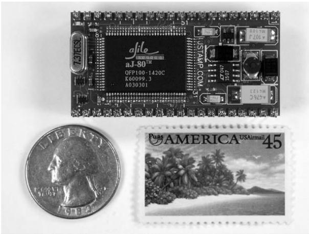
Fig. 5. Systronix JStamp Processor
