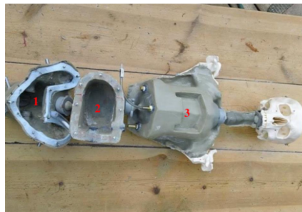
Figure 1 A TCCC mannequin, (1) electronic control compartment, (2) blood pumping housing, (3) blood reservoir
