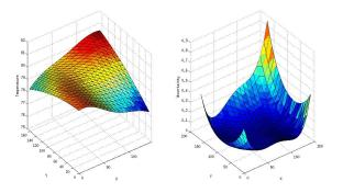
Fig. 3. Temperature model of actual lab space, mean (left) and variance (right). Values displayed are on the horizontal plane, midway between the ceiling and floor.
