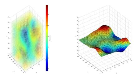
Fig. 2. Point cloud displaying simulated temperatures (left). Temperature on horizontal plane, midway between the ceiling and floor (right).
