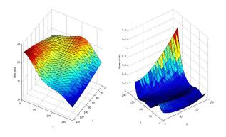
Fig. 4. Humidity model of actual lab space, mean (left) and variance (right). Values displayed are on the horizontal plane, midway between the ceiling and floor.
