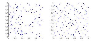
Fig. 1. Uniform random points (left) versus points from the Halton sequence (right).
