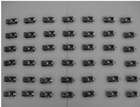
Figure 10: Layout of 42 X-bow T-Sky Motes.
