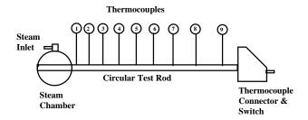
Figure 8: Layout of the Heated Rod Experiment.
