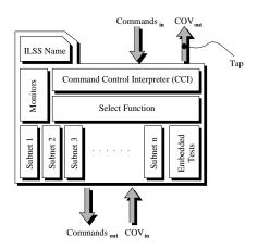
Figure 12: Instrumented Logical Sensor Module.
