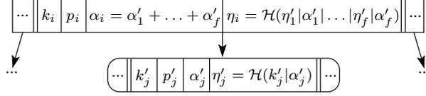
Fig. 4. The AAB-tree. On the top is an index node. On the bottom is a leaf node.  $k_i$  is a key,  $\alpha_i$  the aggregate value,  $p_i$  the pointer, and  $\eta_i$  the hash value associated with the entry.
