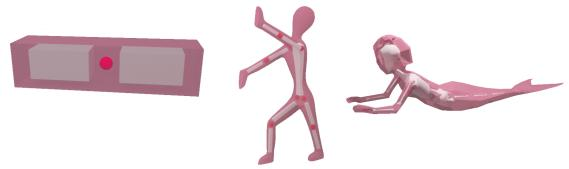
**Figure 5: Visualization of the interior of our models.** The deformable and rigid components are colored using pink and white respectively. The joints are illustrated using red dots.
