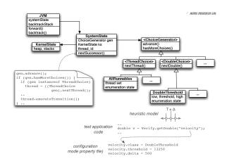
Figure 13: Choice generators as a means of implementing RTSJ scheduling.
