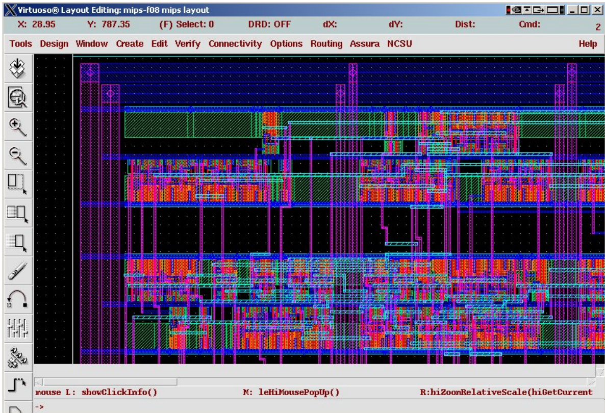
Figure 13.13: Layout of flat MIPS core (zoomed view to show standard cell rows)
