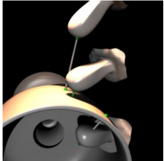
Figure 2: Virtual proxies are important in the penetrating case. The maximal distance is required by the haptics tracing algorithm. Global solution discontinuities such as “chopping through” an object are not desirable. Because the velocity formulation (shown) is the “most local,” it is the method of choice for the penetrating case.
