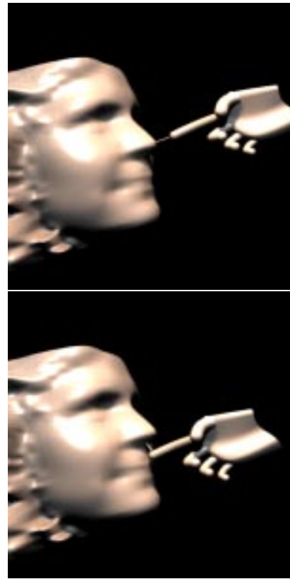
Figure 4: Combined global monitoring and local parametric tracing enable surface-surface contact analysis at kilohertz rates for haptics control.
