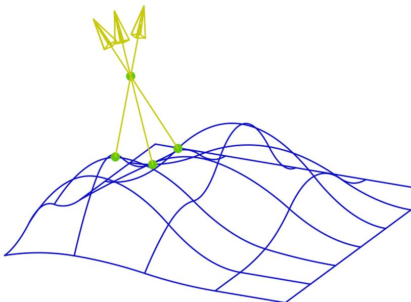
**Figure 33: All local minimum distance solutions are found using the normal cone approach. Nodal mapping and Newton's method improve the final solution.**
