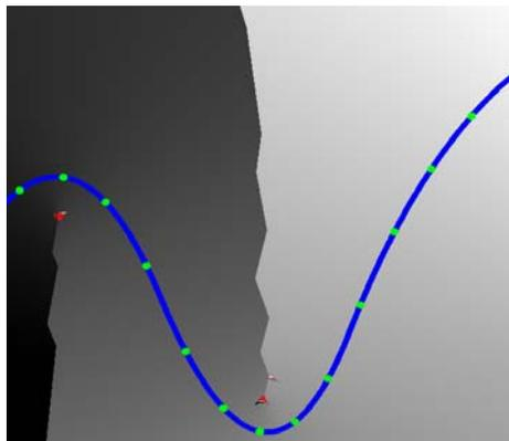
**Figure 20: Choosing a seed point that converges only to a local minimum produces the zigzag pattern along the medial axis of the curve.**
