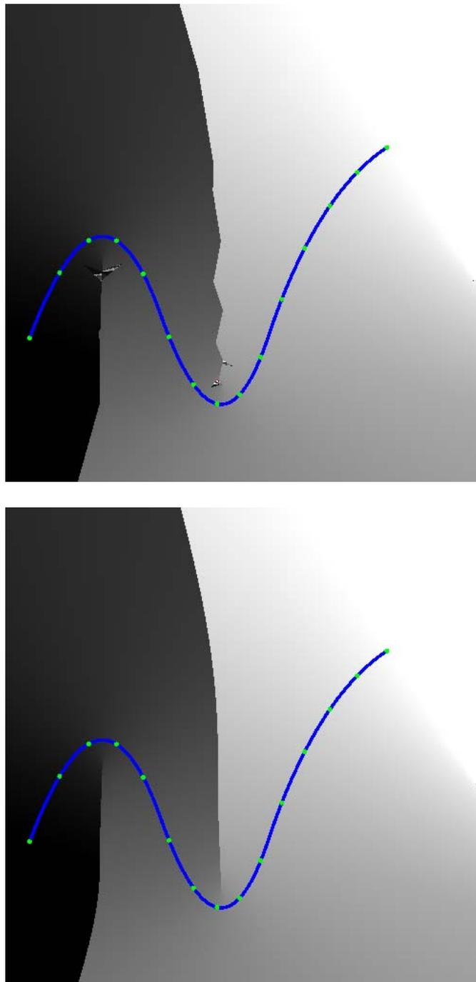
**Figure 24: Distance fields computed using a single seed point and using lower bound pruning. (top) Only using the closest seed point yields incorrect global minima. (bottom) The lower bound pruning technique developed in this chapter produces global minima as well as improved convergence.**
