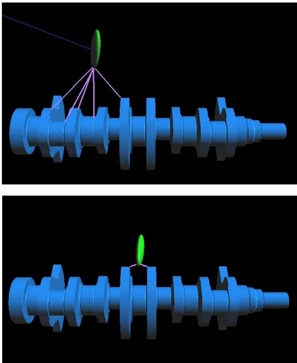
**Figure 49: Finding all LMDs will create forces between far apart portions of the models, as shown in the top image. Using a small cutoff distance in the lower image removes unnecessary LMDs from consideration and controls the onset of forces.**
