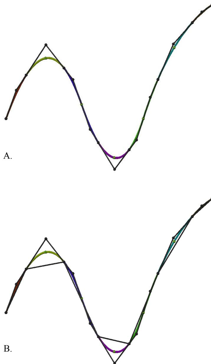
**Figure 22: A refined curve provides a separate convex hull for each seed point. (A) The interval associated with each seed point colors each portion of the curve. (B) The refined control polygon produces tighter convex hulls that more closely bound the seed points.**
