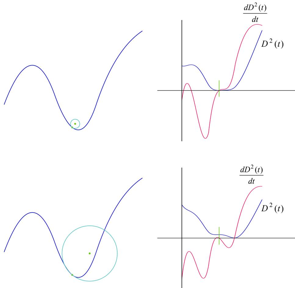
**Figure 4:** As the query point moves away from the curve (left column), the squared distance function (right column) changes from a minimum to an extremal distance at the same zero crossing of the derivative function.
