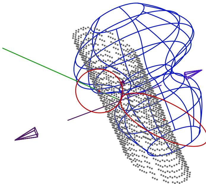
**Figure 30: A cylindrical ellipsoid degeneracy quadric forms from a point on a surface of revolution.**
