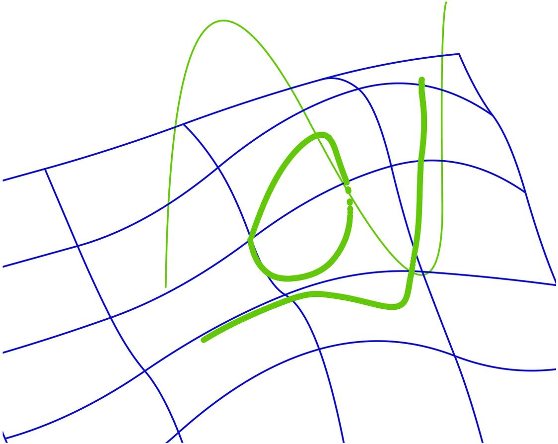
**Figure 35: The query point moves along the test path (thin line). The local closest points on the surface are shown as densely placed points, and include regions where three local minima were found. This type of test is sped using a dynamic subdivision tree.**
