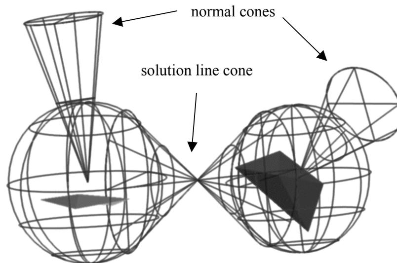
**Figure 43: The solution line cone now spans between the two bounding spheres – encompassing all possible solution lines between the models.**
