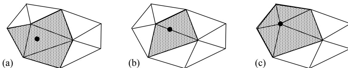
**Figure 55: The three possible neighborhoods to be checked depend on the minimum distance point from the last time step. In (a), the minimum distance point was on a triangle face, and it and all its adjoining triangles form the neighborhood. When the point from the previous step was on an edge, as in (b), the triangles that share that edge form the neighborhood. The final case (c) is for a vertex, where all triangles that share that vertex form the neighborhood.**
