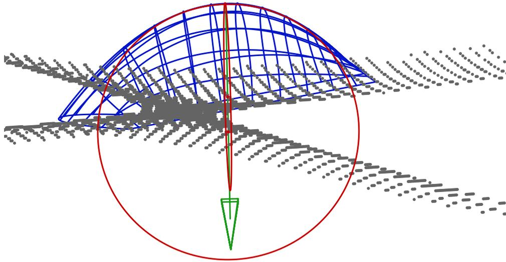
**Figure 28: The surface normal intersects the degeneracy quadric at the radius of curvature for each the principal curvatures.**
