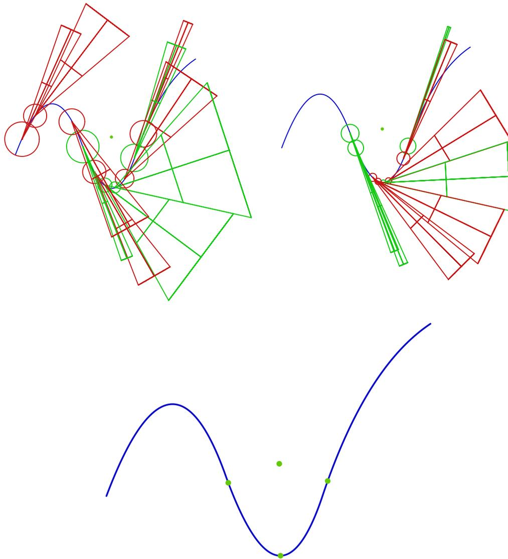
**Figure 26: Two consecutive levels of subdivision during the normal cone approach and the final result are shown. The cones are the tangent cones computed from the derivative curve and the circles provide the basis for solution line cones. Intervals in that pass are subdivided and ones that fail are removed from further computation.**
