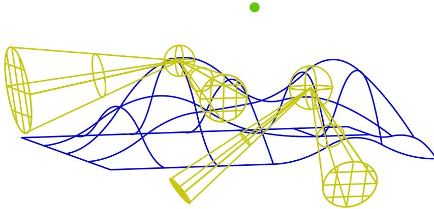
**Figure 31: Two surface patches with their sample tangent cones. The spheres bound the spatial extent of the patch and help to form the solution line cone from the query point.**
