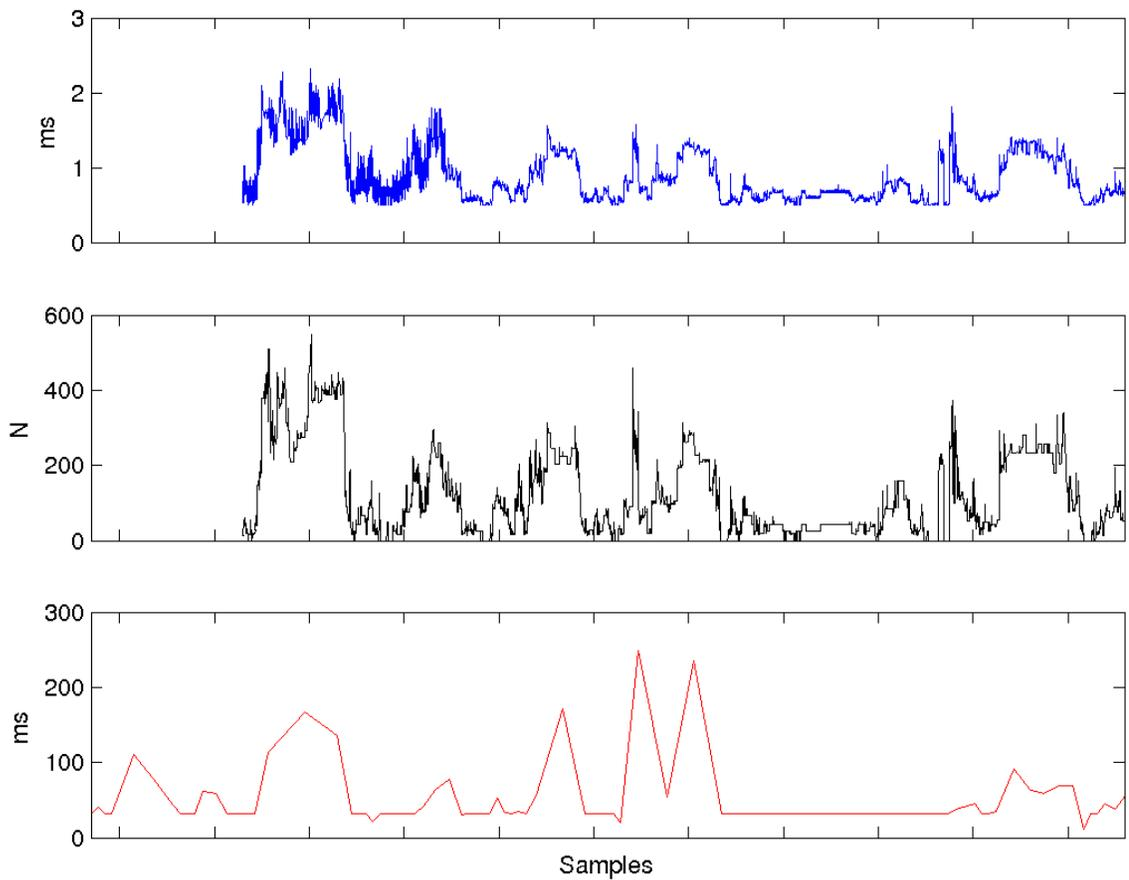
**Figure 57: The crankshaft model has 45,000 triangles and the gear has 6,300 triangles. The local update time correlates well with the number of triangles searched. The bottom graph shows the computation time for the global search to find the LMDs. Without the local update, haptic interaction would have been unstable and slow.**
