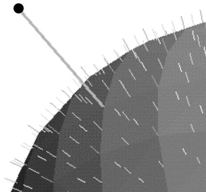
**Figure 39: The line between the query point and the feature is in line with the normal at the feature.**
