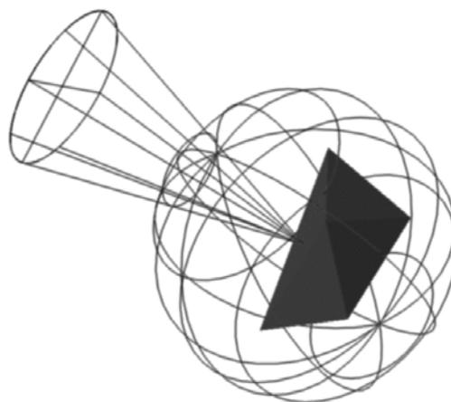
**Figure 38: The spatialized normal cone encompasses the range of normals and bounds the geometry.**
