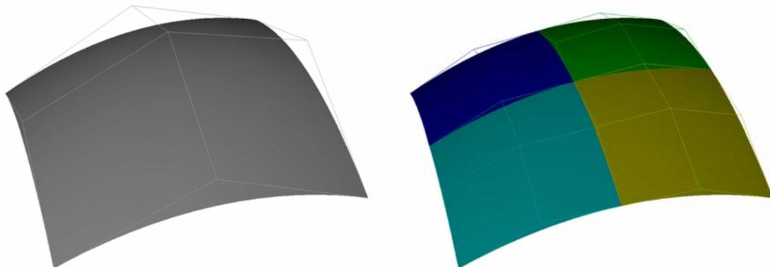
**Figure 32: Refining a patch splits it into four independent surfaces. The new control meshes more tightly bound the surface.**
