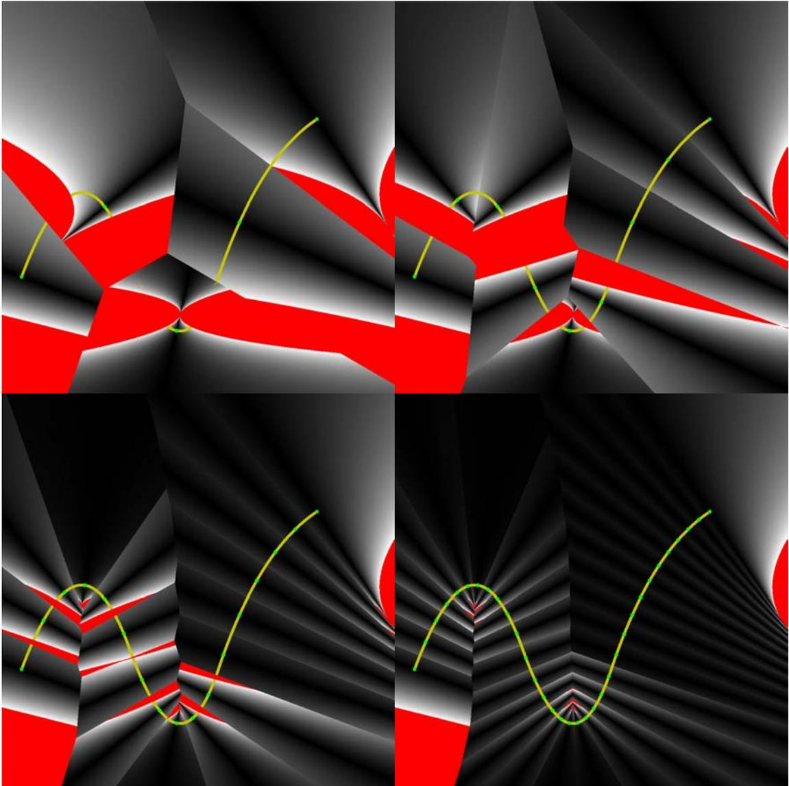
**Figure 10: Regions of  $|G'| \geq 1$  are easily visualized by finding the closest seed point on the curve to each pixel and computing the value of  $G'$  based on the intrinsic properties of the curve. Magnitudes larger or equal to one are colored. The images above show visualizations of  $G'$  based on varying numbers of seed points.**
