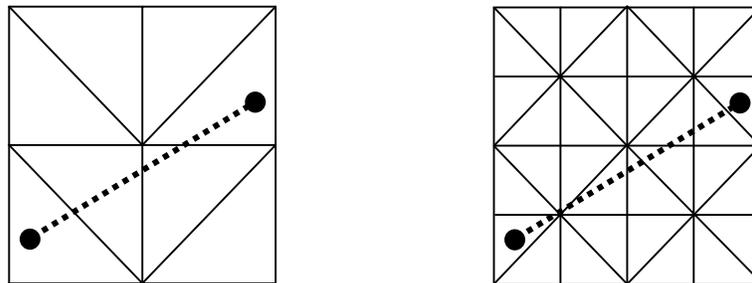
**Figure 56: The number of triangles crossed grows roughly by  $\sqrt{n}$ , where  $n$  is the number of triangles in the model. (a) This model has eight triangles and four are crossed. (b) There are four times as many triangles in this model, but roughly twice as many are crossed.**
