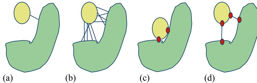
**Figure 48: Different distance possibilities for force computation. (a) The global minimum distance. (b) All pairs within a distance. (c) Contact points between two colliding models. (d) Local minimum distances.**
