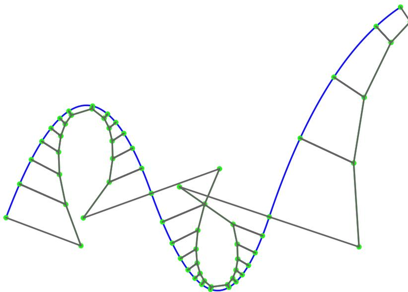
**Figure 18: A tighter bound requires fewer seed points than for the bound in Figure 17.**
