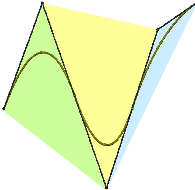
**Figure 21: This quadratic curve has three polynomial pieces. The convex hull for each piece is shown as a different filled region. Each convex hull can enclose multiple seed points.**
