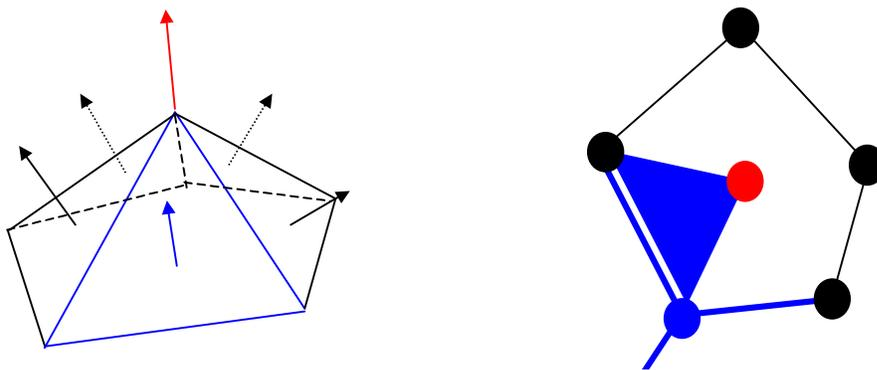
**Figure 42: A. The vertex normal is surrounded by triangles. B. Each triangle normal maps to a point on the Gauss sphere and each edge maps to an arc.**
