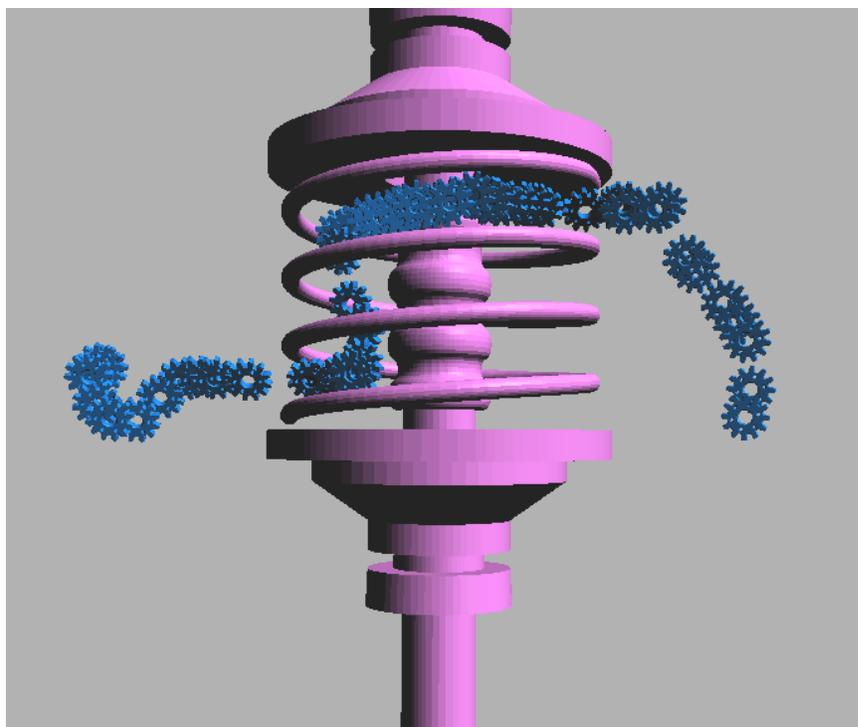
**Figure 62: The gear had to rotate to slip between the coil and center axis of the environment model.**
