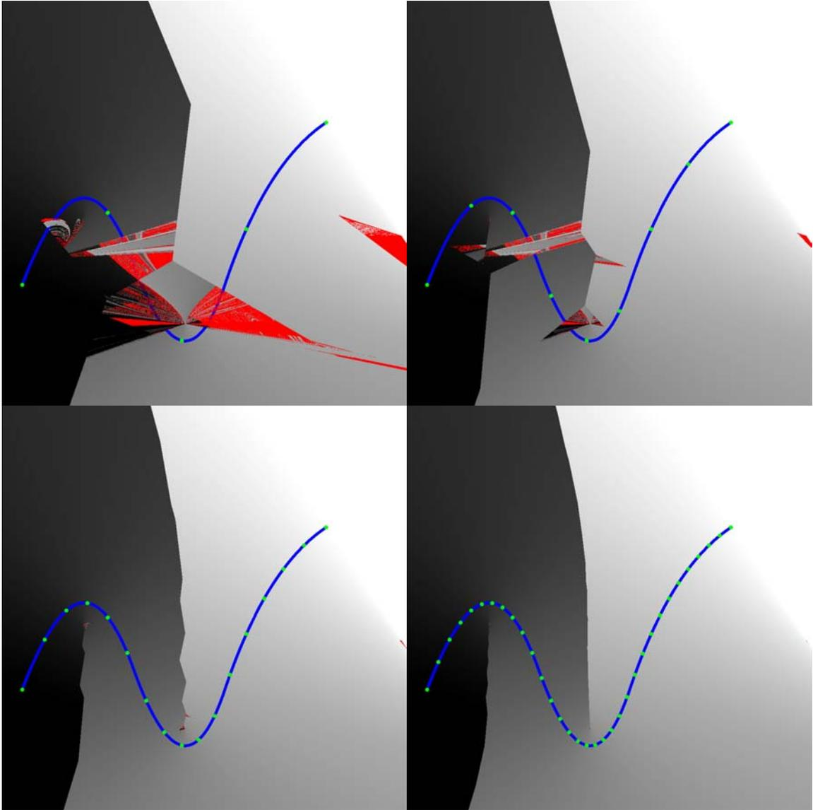
**Figure 9: Closest point maps set pixel intensity to the parametric value of the closest point on the curve. This mapping provides more information about where the standard algorithm converged to than the distance map.**
