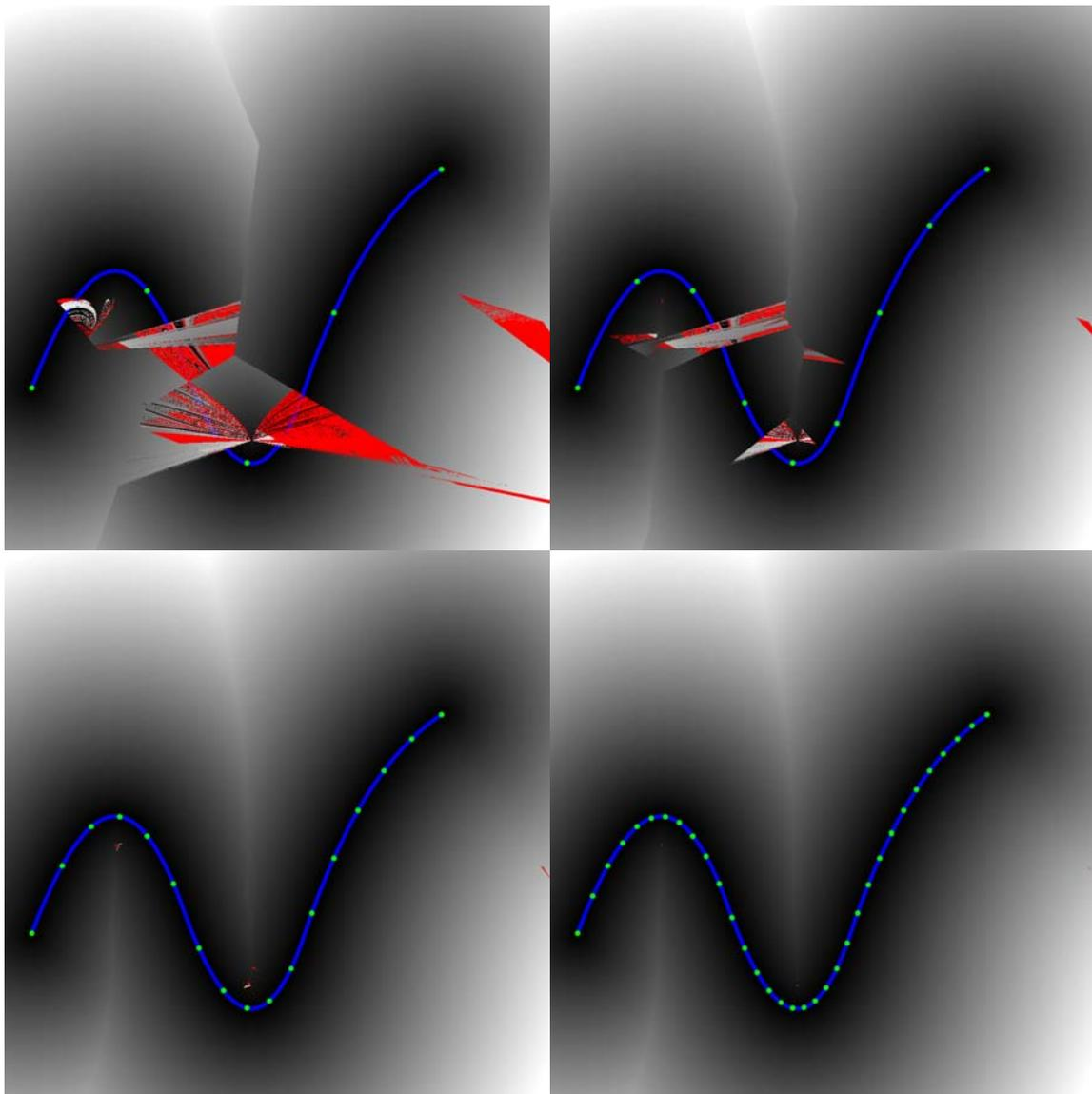
**Figure 8: Distance maps show distance to the curve by mapping pixel intensity to distance. The number of seed points is increased in each successive image, and places where Newton's method fails to converge map to a warning color.**
