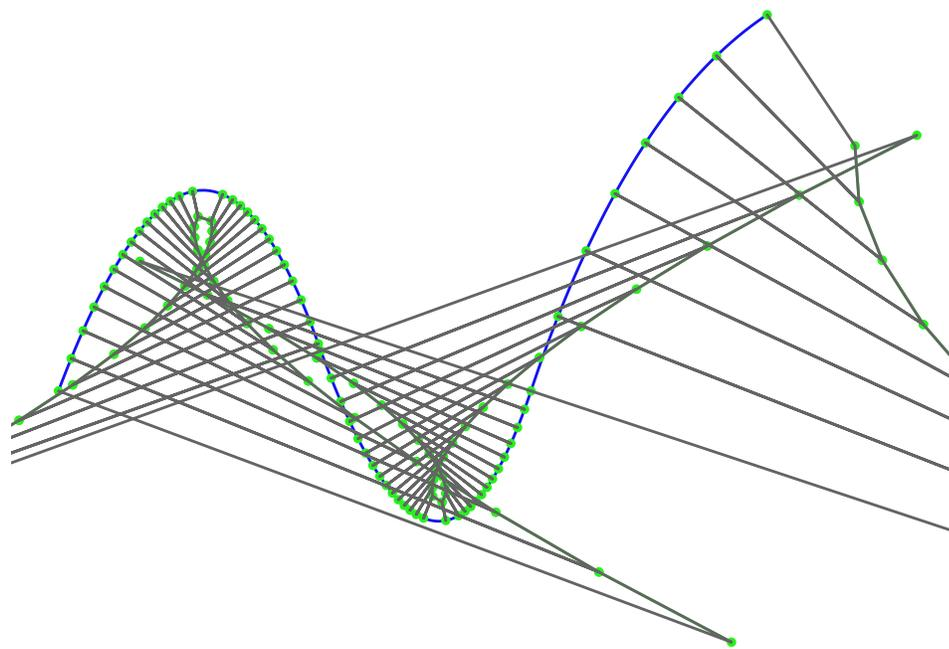
**Figure 17: A sample curve with its approximate scaled evolute bound and generated seed points.**
