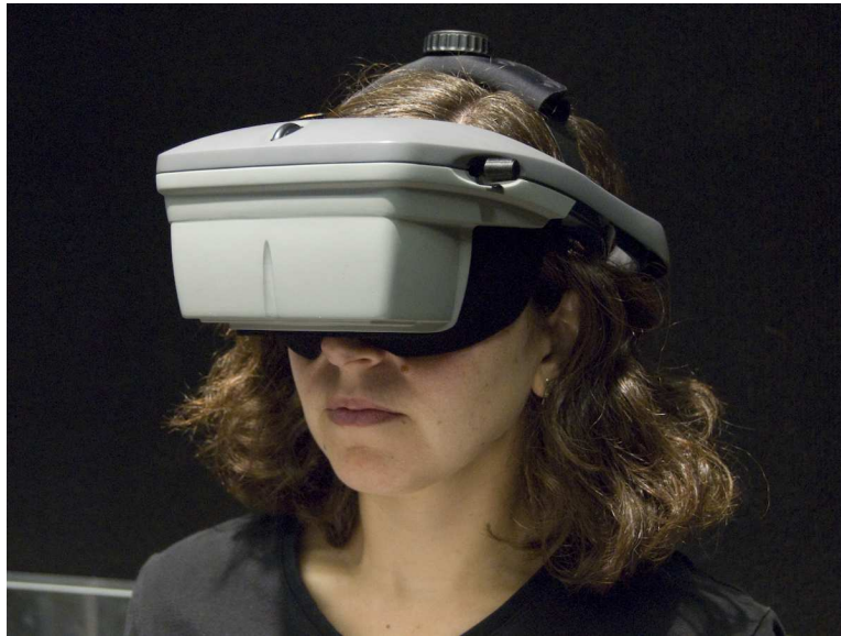
Fig. 3. NVIS nVisor SX head-mounted display, which was used in the HMD conditions. Not shown in the figure is a neck collar used to occlude the area around the feet in order to avoid a potential confound when the body is not visible in the HMD conditions [Creem-Regehr et al. 2005].
