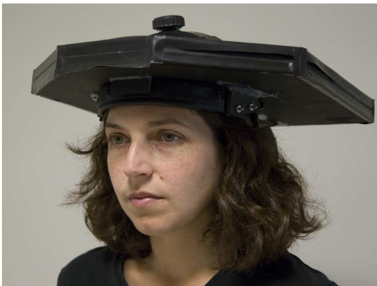
Fig. 5. Inertial band, with similar mass and moments to the real and mock HMDs, but without field of view restriction or a sense of “wearing a helmet”.
