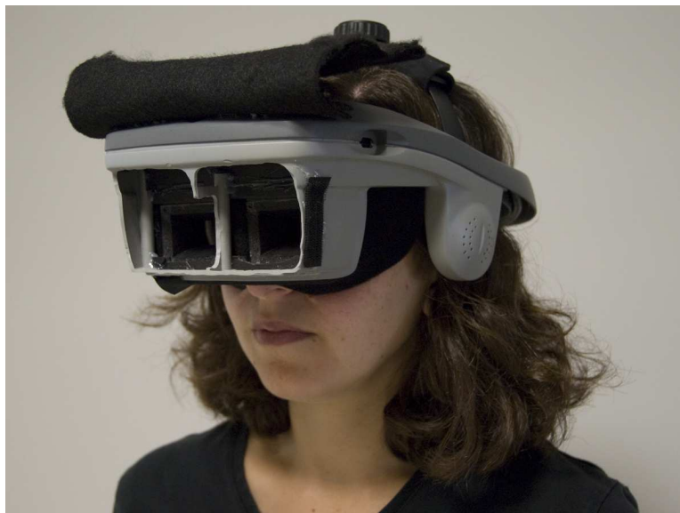
Fig. 4. Mock HMD based on NVIS nVisor SX HMD shell used during real world viewing conditions. As with all of the other conditions the neck collar was used to restrict subjects from looking at their feet or the floor in the immediate vicinity of where they were standing.
