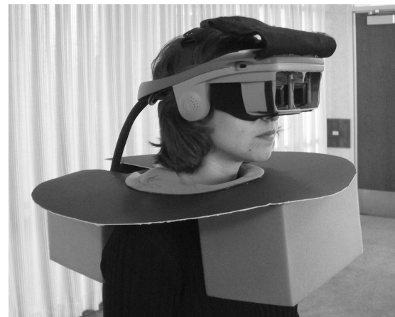
Figure 2: Mock HMD based on NVIS nVisor SX HMD shell used during real world viewing conditions. A neck collar is used to occlude the area around the feet.
