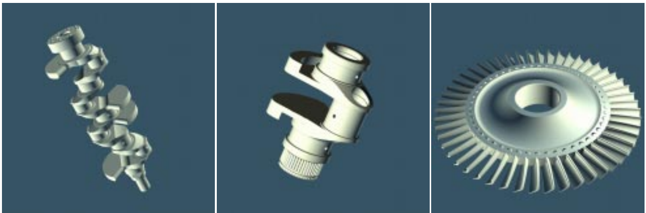
Figure 10: Mechanical parts produced by the Alpha_1 [11] modeling system (crank, Crank1A, and allblade).
