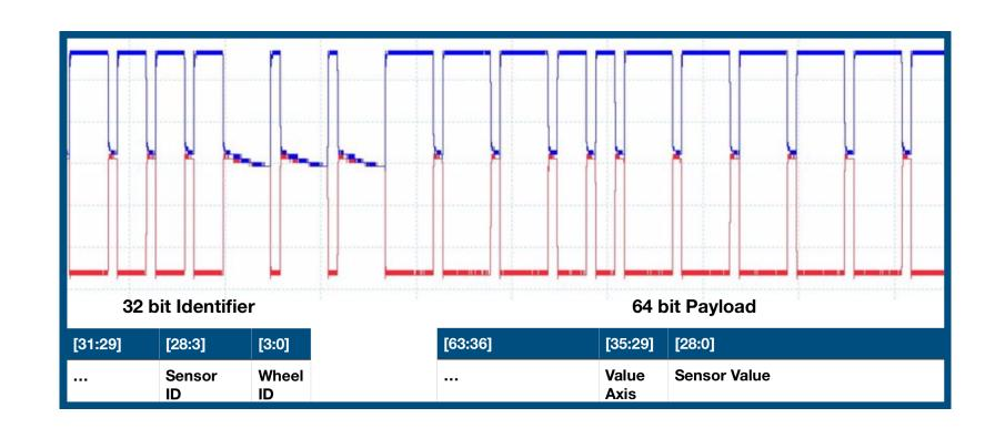
Via the CAN protocol, DRAGLINE supports sensors such as car speed, accelerator pedal position, brake pedal position, rotations per minute, steering angle, three axes of velocity and much more.
