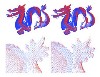
Figure 3. Dragon scans at  $0^{\circ}$  and  $48^{\circ}$  with M in blue and D in red, registered using FICP (top left) and ICP (top right). Zoomed images of the alignment around dragon's tail with FICP (bot. left) and ICP (bot. right) demonstrate the skew in the alignment due to ICP.
