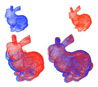
Figure 2. bunny: M in blue (top left) and D in red (top right) with Deform noise with  $p_I=.75$ . Registered using FICP (bottom left) and ICP (bottom right).
