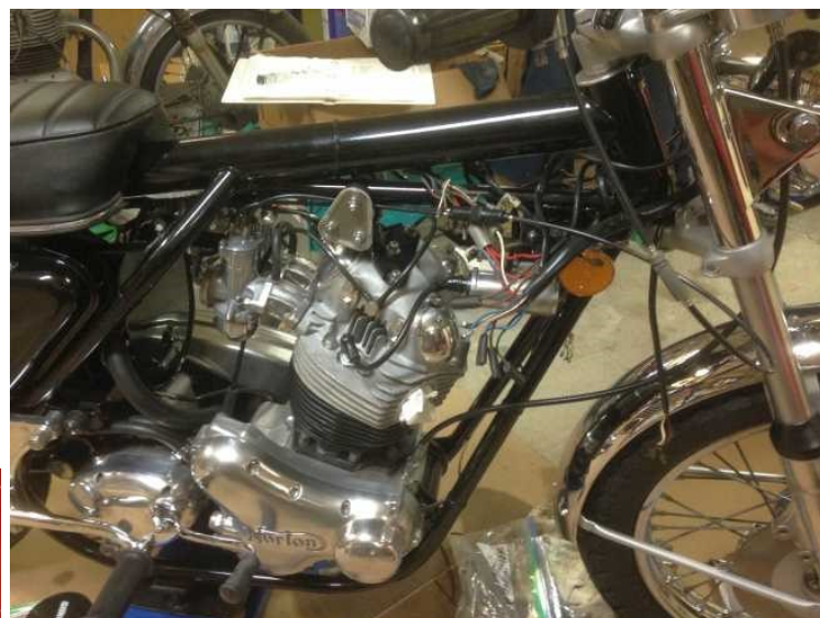
Norton engine and wiring back in frame
