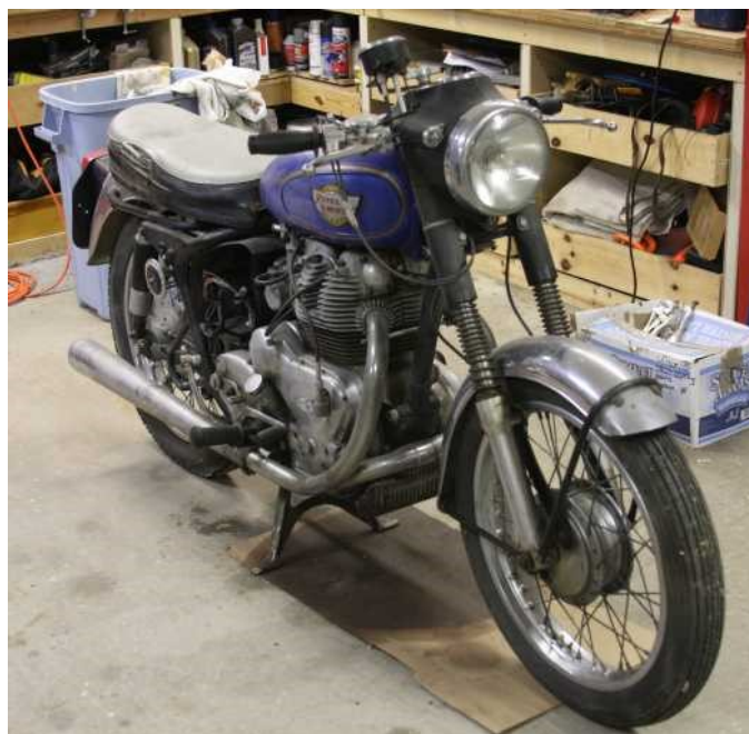
Enfield before teardown - wrong tank and missing side covers
