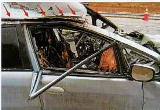
A Texas jury concluded that substandard roof repairs to this used 2010 Honda Fit aggravated the effects of a collision in December 2013. Red arrows show where roof detached during the crash.
