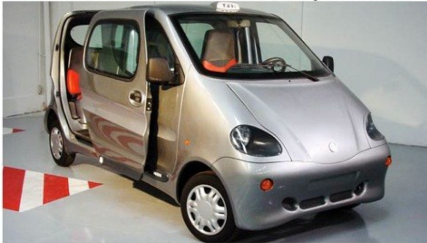
This six-seater tax, which should be available in India next year, is powered entirely by a tank filled with compressed air.
